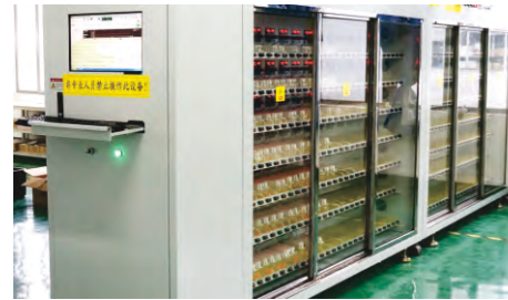
LED Driver Aging Testing Equipment
