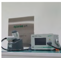
Electrostatic Discharge System
